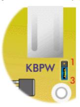
Figure 3 - 3 : Keyboard Power Jumper
